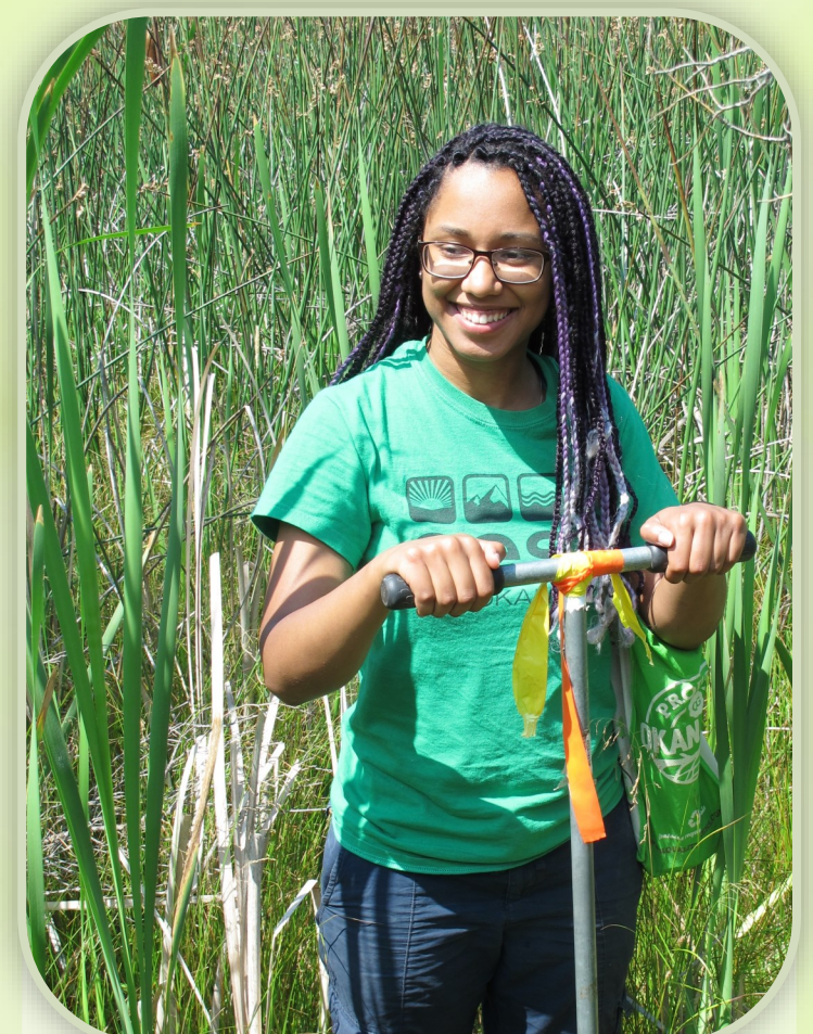
Sampling wetland soil using an auger
